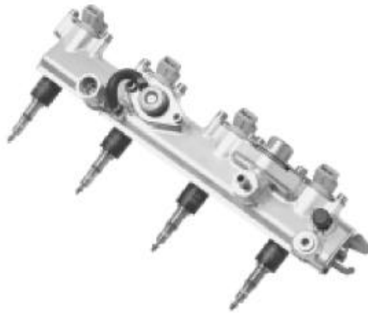
Development of Fuel System Assembly
